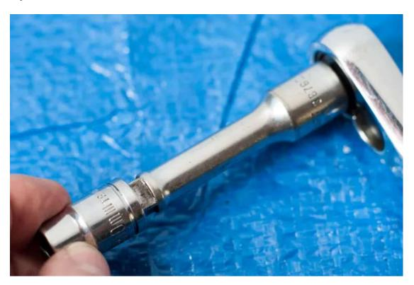
Place the socket that matches the nylon lock nut onto the 3/8-inch drive ratchet.
