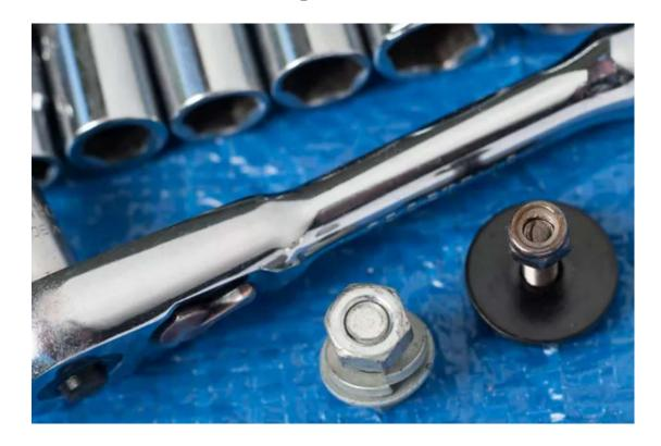
Nylon lock nuts differ from a standard hex nut in that they have a nylon insert secured within the nut. The nylon insert is located in a tapered section located at the back of the nut. When you install the nylon lock nut onto a bolt or threaded stud, the nylon insert wraps around the threads and locks the nut in place. This gives a nylon lock nut a distinct advantage over a lock washer when the bolt or threaded stud is subject to vibration, as the nylon lock nut is unaffected by vibration.
