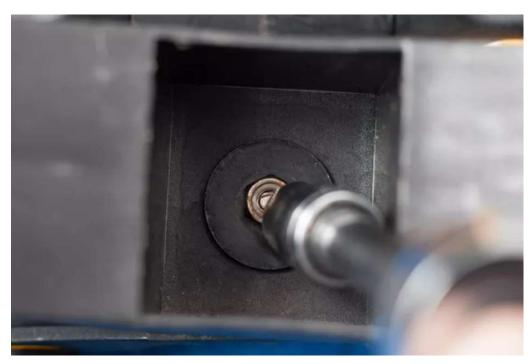
Slide the socket onto the nylon lock nut and turn the handle of the ratchet clockwise to turn the nylon lock nut onto the fastener. You will feel some resistance from the nylon lock nut as you turn it onto the fastener. This is created by the nylon insert and is completely normal.
